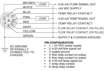
Note: For pulse output, the flow relay contact is closed for 3 msec (pulsewidth)
